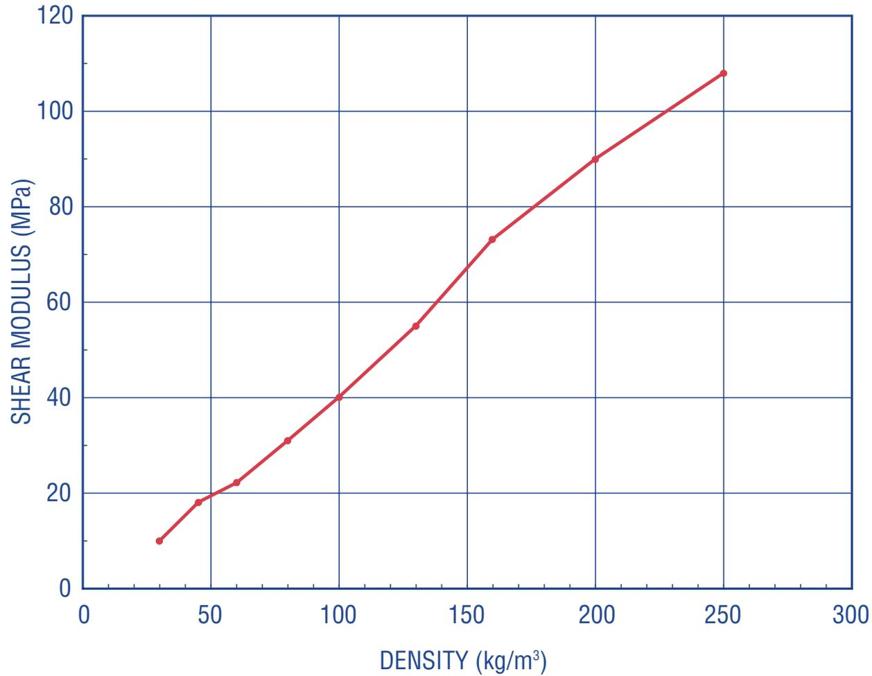
Shear modulus at +23°C as a function of density according to ASTM C 273 and ASTM D 1622.
