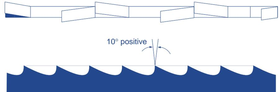
Figure 7. Band-saw blade, top and side view.
