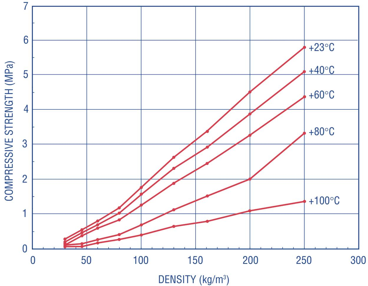
Compressive strength perpendicular to the plane at +23°C and +100°C as a function of density acc. to ASTM D 1621 and ASTM D 1622.
