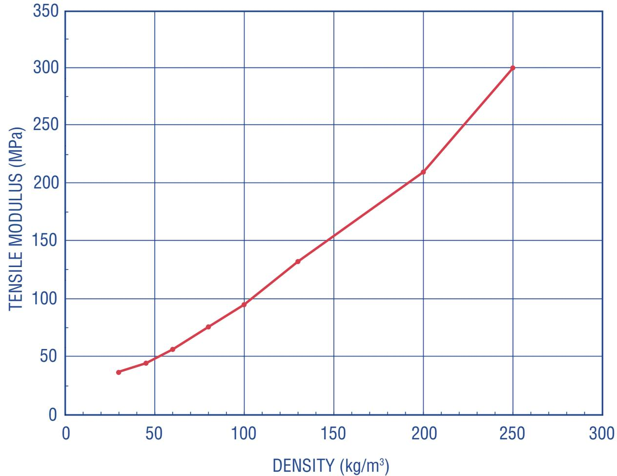
Tensile modulus parallel to the plane at +23°C as a function of density according to ISO 1926 (extensometer) and ASTM D 1622.
