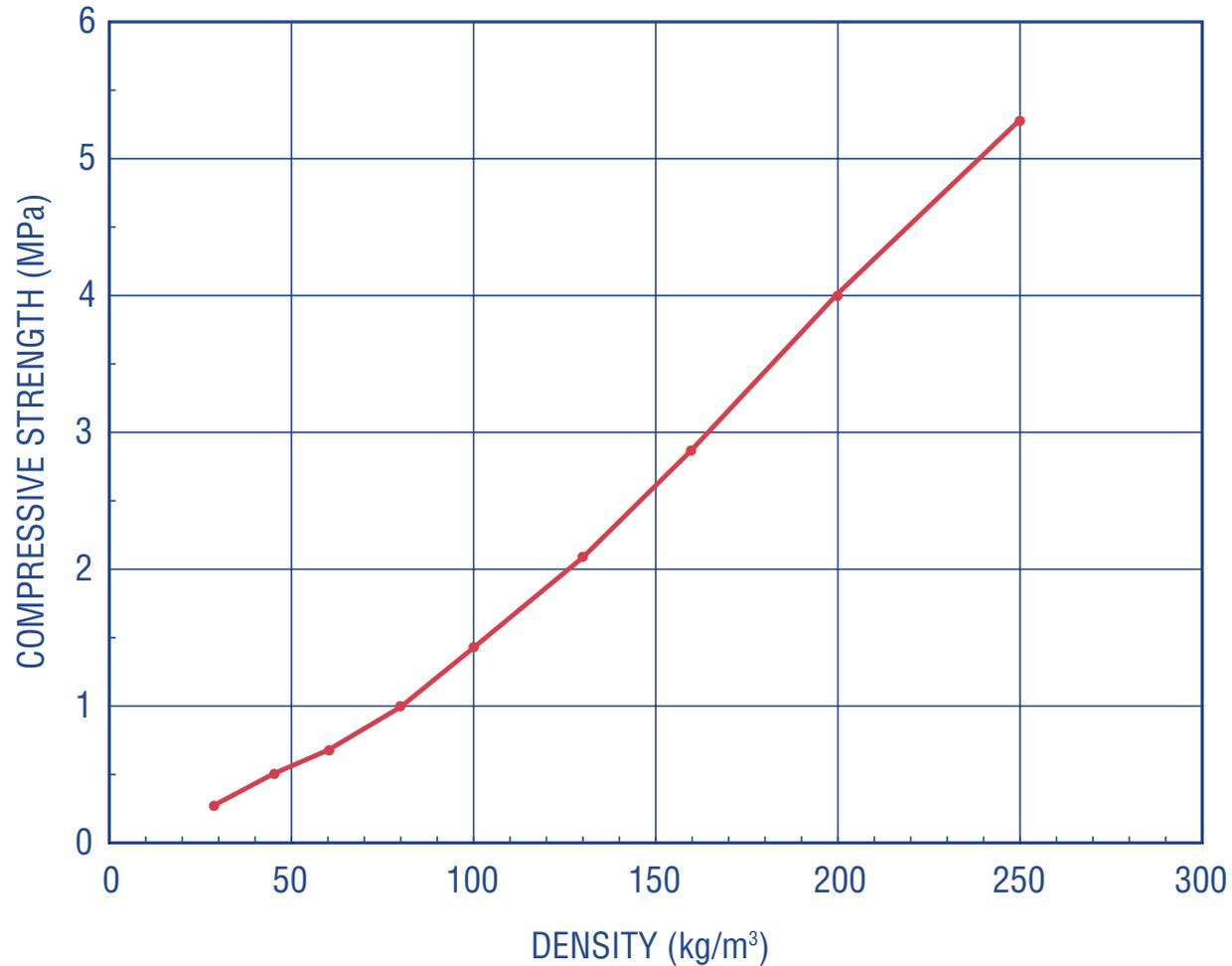
Compressive strength parallel to the plane at +23°C as a function of density according to ASTM D 1621 and ASTM D 1622.
