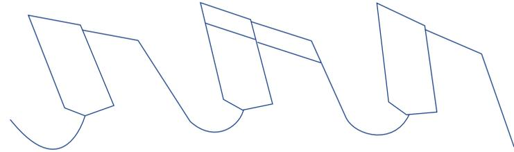
Figure 2. Alternately sharpened blade, side view.
