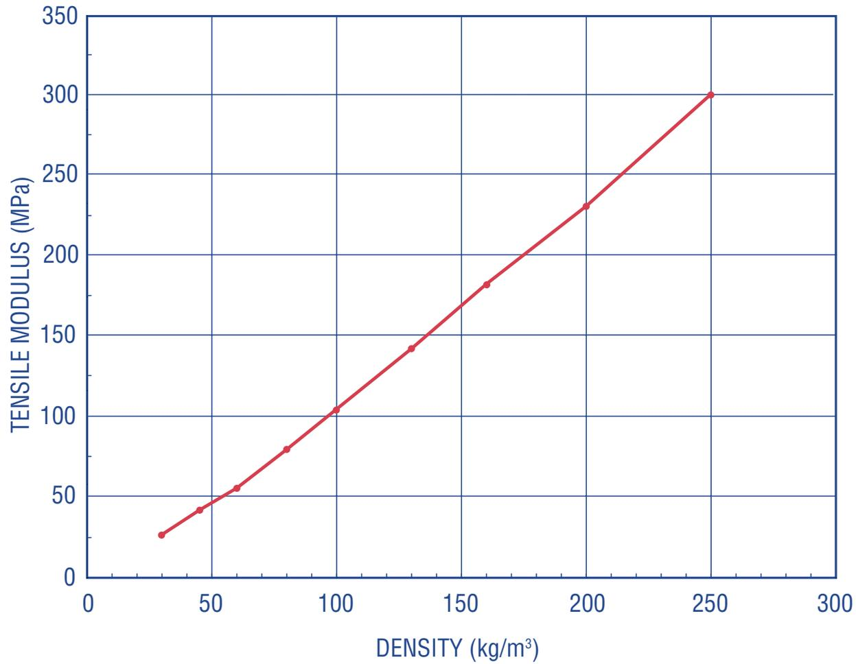
Tensile modulus perpendicular to the plane at +23°C as a function of density according to ASTM D 1623, ASTM D 1621 procedure B and ASTM D 1622.
