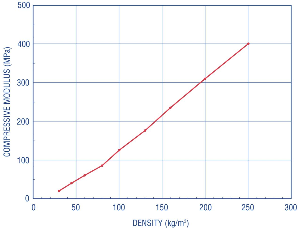
Compressive modulus perpendicular to the plane at +23°C as a function of density according to ASTM D 1621 (extensometer) and ASTM D 1622.
