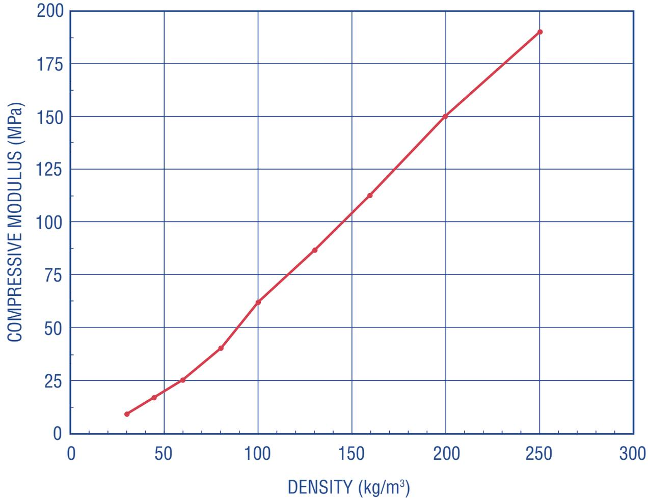
Compressive modulus perpendicular to the plane at +23°C as a function of density according to ASTM D 1621 (crosshead movement) and ASTM D 1622.
