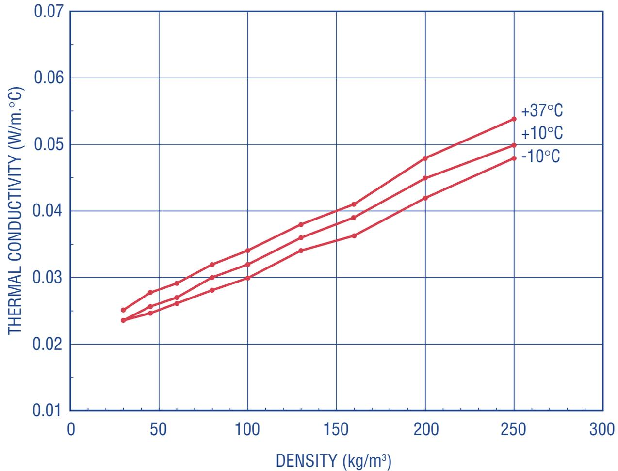
Thermal conductivity at -10°C, +10°C and +37°C as a function of density according to ASTM C 177 and ASTM D 1622.
