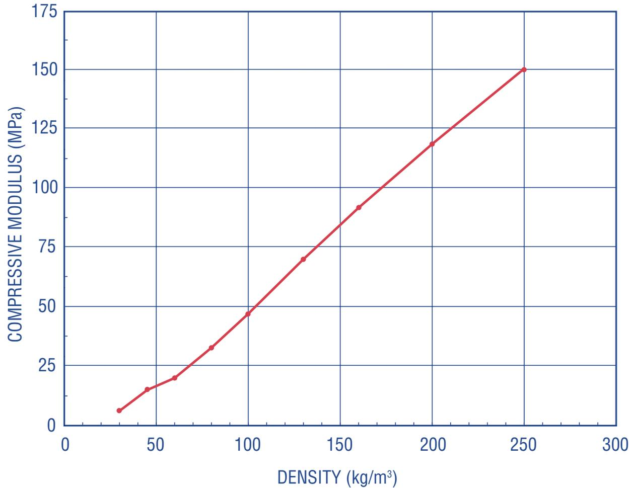
Compressive modulus parallel to the plane at +23°C as a function of density according to ASTM D 1621 (crosshead movement) and ASTM D 1622.
