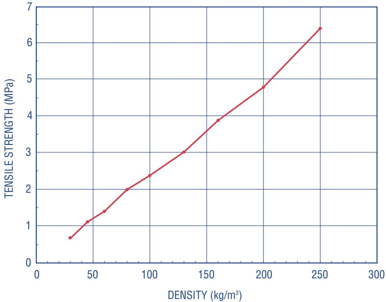
Tensile strength parallel to the plane at +23°C as a function of density according to ISO 1926 and ASTM D 1622.
