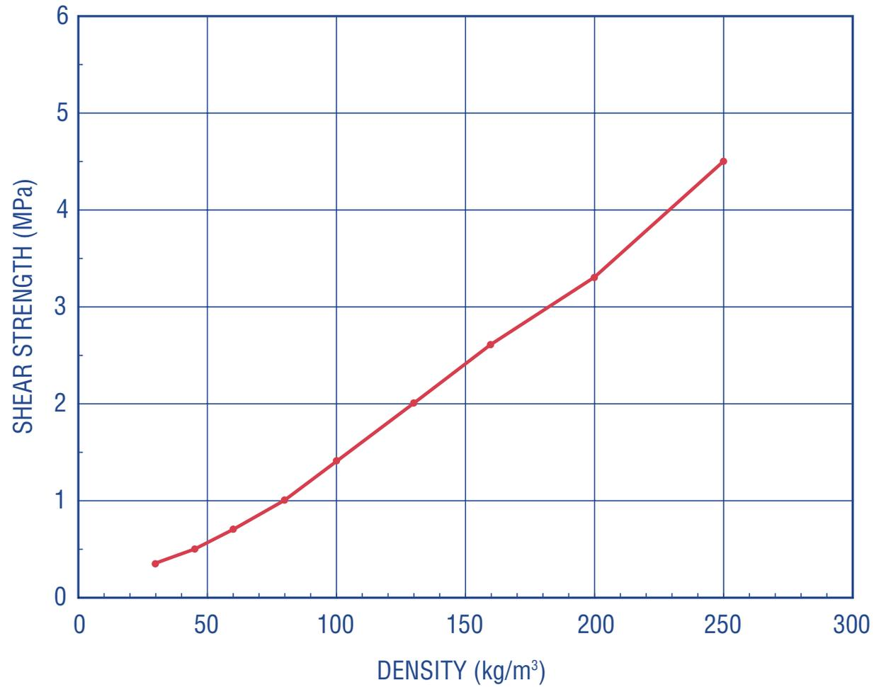
Shear strength at +23°C as a function of density according to ASTM C 273 and ASTM D 1622.
