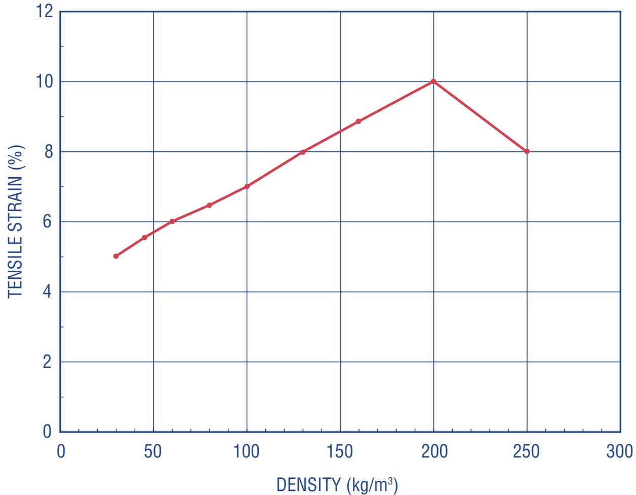
Tensile strain parallel to the plane at +23°C as a function of density according to ISO 1926 (extensometer) and ASTM D 1622.
