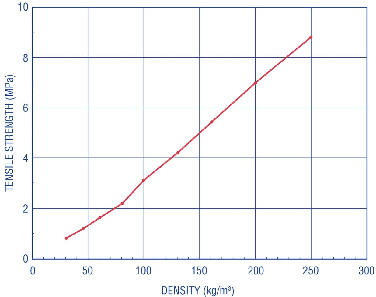
Tensile strength perpendicular to the plane at +23°C as a function of density according to ASTM D 1623 and ASTM D 1622.
