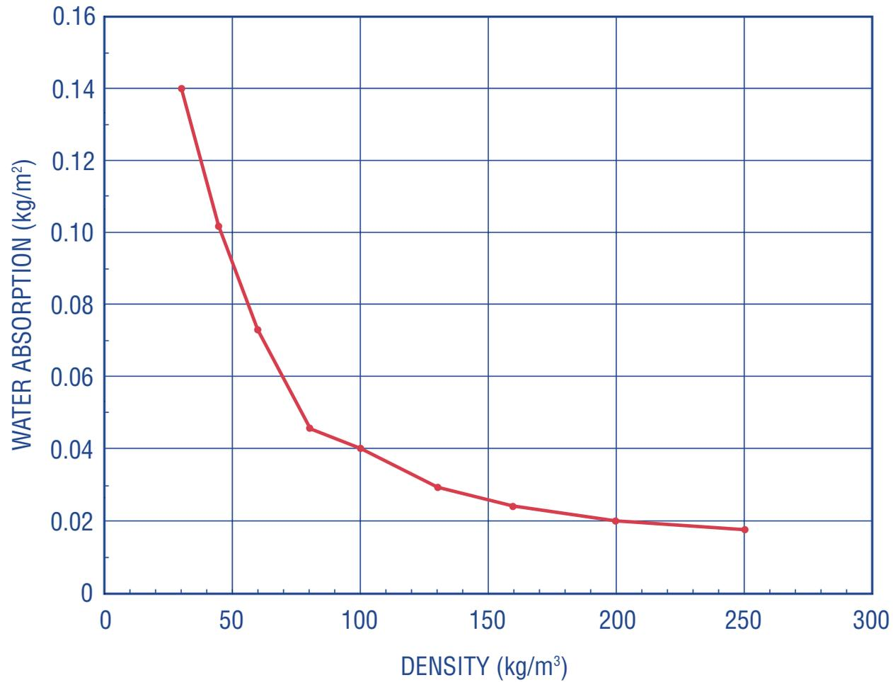
Water absorption at 23°C as a function of density
