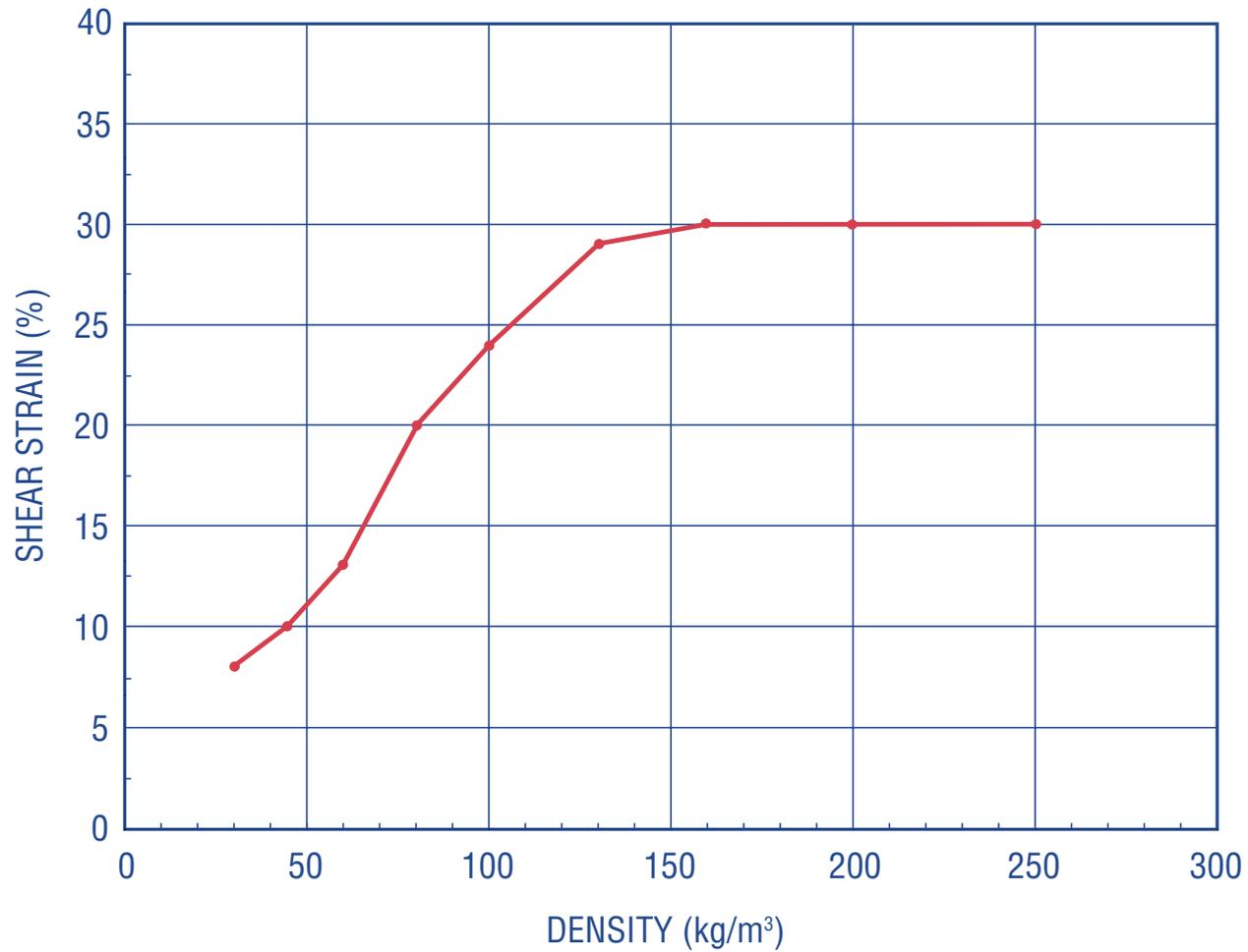
Shear strain at +23°C as a function of density according to ASTM C 273 and ASTM D 1622.
