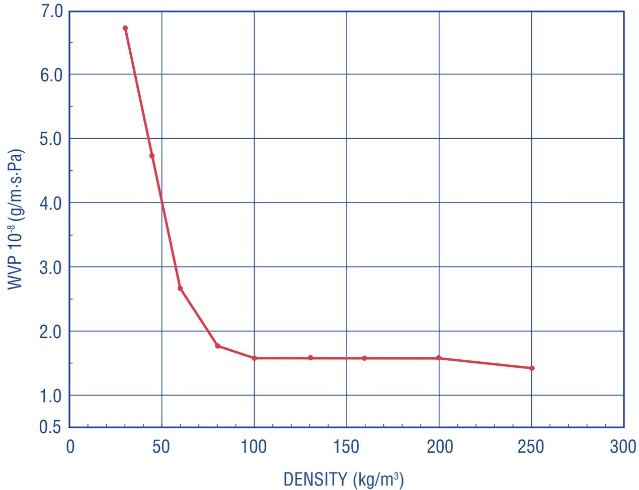
Water vapour permeability at 22°C as a function of density
