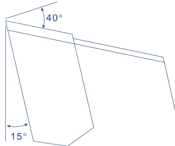
Figure 4. Trapezoidally sharpened blade, side view.
